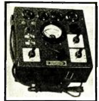
Latest emission-type tube tester makes hot emission tests of all types of tubes. (1299)
