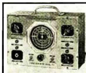
A wide-range oscillator with continuous range of fundamentals from 125 kc. to 16 mc. (1297)
