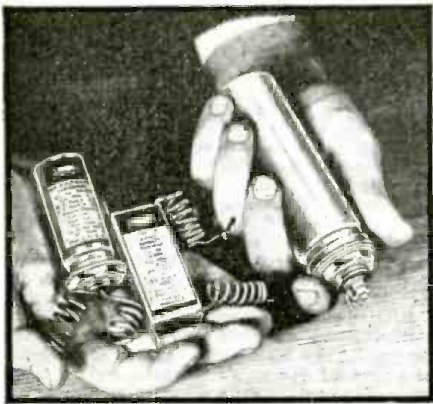
The new "etched-foil" electrolytics. (1301)
